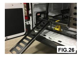
6.22 Attach the bumpers to the ramps. Position the bumpers so the doors contact them when they are closed. (FIG.27&28)
