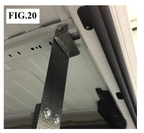
6.19 With the top deck lowered, align the rear of the deck correctly over the lower deck, then tighten the 4 fasteners that tie the roof brackets to the front legs. (FIG.22&23)
