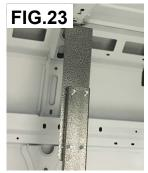
6.20 Adjust the actuator to the correct position (Suggestion: Place a 1" thick spacer between the decks with the actuator fully extended) and tighten the 4 actuator bolts. (FIG.24)
