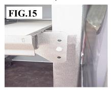
**NOTE:** Use middle hole for low roof vans, and the bottom hole for high roof vans the top hole may also be used on low roof vans where more room is necessary on top. The bearing in the lift arm will need to be moved to the corresponding hole. **(FIG.16)**
